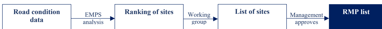
Figure 10. Process for selecting sites to be funded from the repair measures of the Transport Administration
