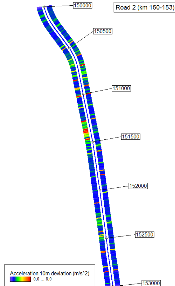
Figure 66_7. Acceleration 10m deviation from section 6 presented as a map.
