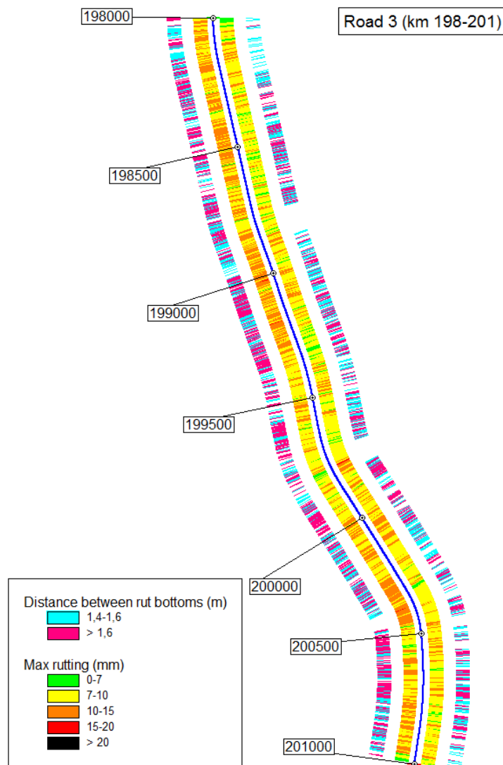
Figure 65_4. Maximum rutting in both lanes (inner lines, colours from green to black) together with distance between rut bottoms (outer lines, colours pink and blue).
