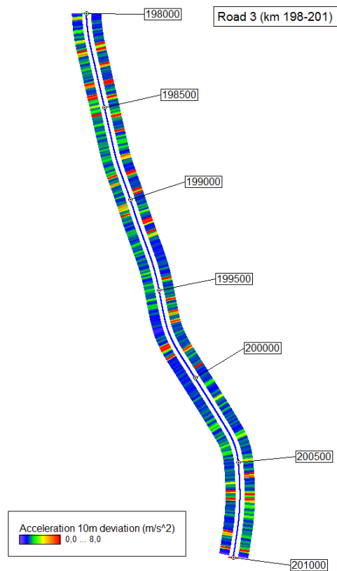
Figure 65_2: Acceleration 10m deviation from section 5 presented as a map.
