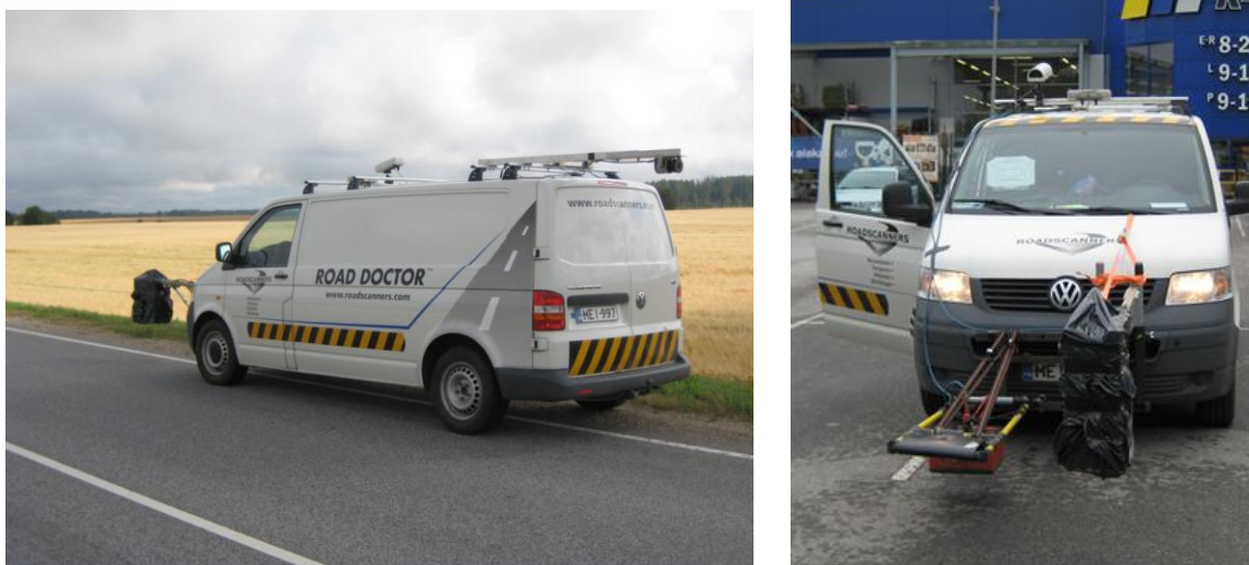
Figure 31_2. The Roadscanners GPR survey system equipped with a 1 GHz air-coupled horn antenna and 400 MHz ground coupled antenna in the front of the vehicle. A video camera is mounted on the roof top with laser scanner.
