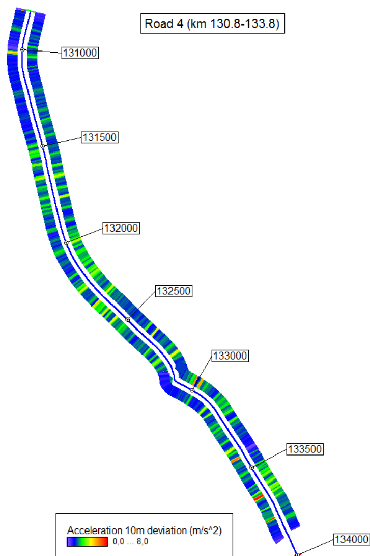
Figure 69_5. Acceleration 10m deviation from section 9 presented as a map.
