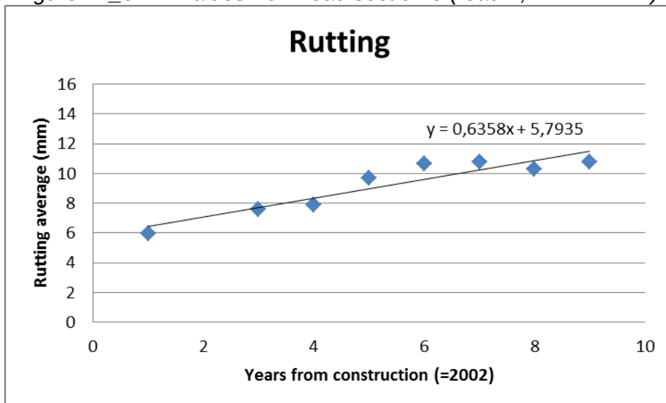
Figure 77_4. Rutting values from road section 8 (road 4, km 144-147).
